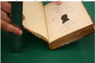
• If there is a drop between where the cover board meets the spine and the surface, measure this drop. This figure becomes **d**.
